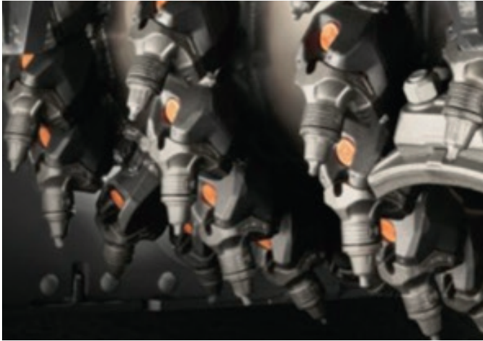
The tool holders with the carbide cutters are clearly visible. The 17 mm Allen bolts are covered by the orange caps.
