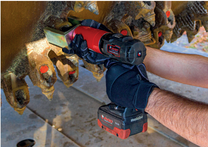
The B-RAD 1400-2 with forked reaction arm on the application.
