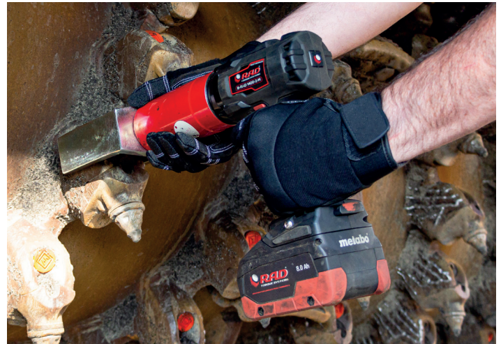
The B-RAD 1400-2 accurately loosens and fastens the bolts to 630 Nm.
