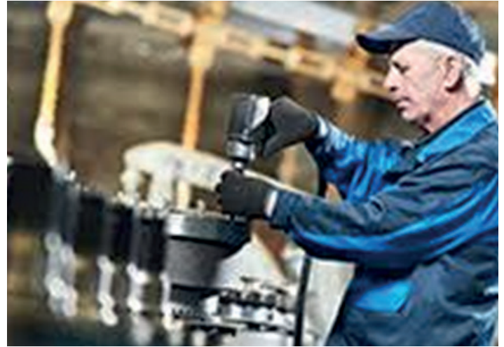
How it used to be done: service with a pneumatic impact wrench.
