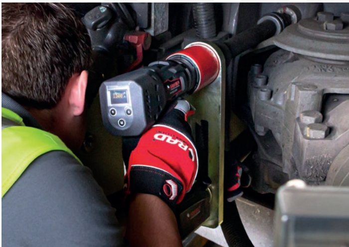
MB-RAD 2000 with sliding reaction arm and double nose extensions.
