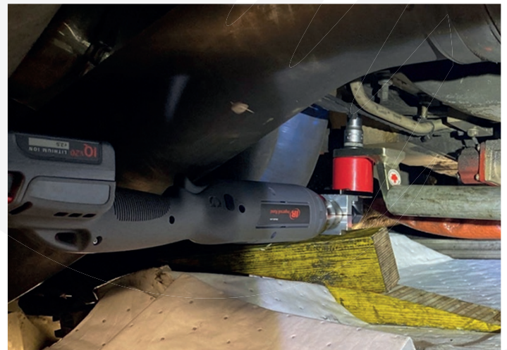
RAD SDM tightening a hard to reach bolt on a train chassis.
