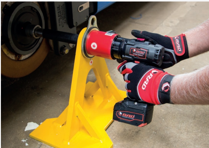
B-RAD SELECT 4000 with special reaction piece on a tram wheel.
