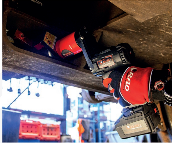
B-RAD SELECT 1400 Offset on bolt with limited space.
