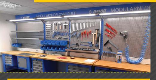
High-quality sheet metal — tool carriages, tool boxes, work benches, tool stands, walls, cabinets, drawers, and all other equipment are made of high-quality sheet metal. It is lacquered so as to protect it against mechanical damages and, if used correctly, practically indestructible.
