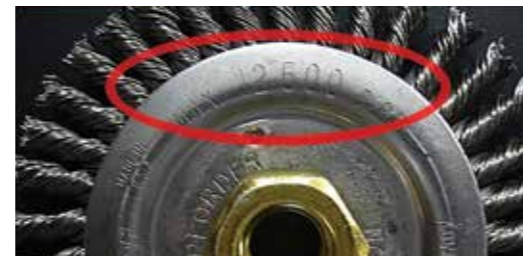
Match the RPM rating of the power brush to the tool being used. The RPM of the tool should never exceed the RPM of the power brush.
