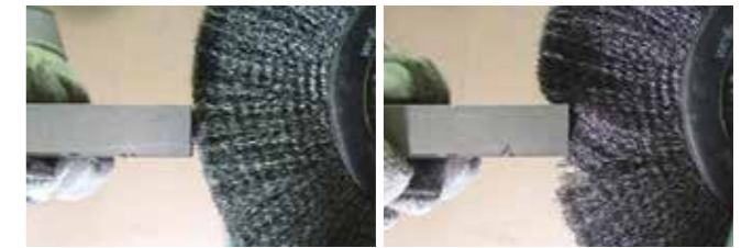
Correct Wire Tips Doing the Work
