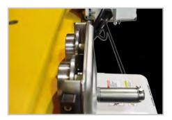
Wheels of both trolleys made of stainless steel
