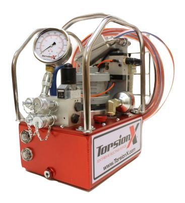
**External Adjustable Pressure Regulator Retract Internal Pressure Relief Valve for Tool Protection** Runs up to 2 Hydraulic Torque Wrenches at One Time **Three-speed High Performance Pump External Adjustable Pressure Regulator** Built in Cooling System Heavy Duty Roll Cage **Remote Control Assembly** 115 volts/60 hz\* 13.1 Amps 1.5 Horsepower 4000 RPM Maximum Oil Flow: 500 Cubic Inches per Minute 2-gallon Oil Reservoir Overall Dimensions: 11.8" x 14.8" x 17.9" Weight (without oil): 60 Pounds
