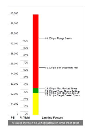
20% Torque: 185 ft lbs Nut Factor: 0.16 60% Torque: 554 ft lbs Socket Size: 2-9/16 in 100% Torque: 923 ft lbs Preload of Stud: 24,000 psi 1 16 17 8 9 12 5 20 13 3 (4) 14 (19) 6 11 10 7 15 18 2 Legacy "Star" Pattern Pass 1: 20% to 30% of Target Torque 1,2,3,4 - 5,6,7,8 - 9,10,11,12 - 13,14,15,16 - 17,18,19,20 • Pass 2: 50% to 70% of Target Torque, Same pattern as Pass 1. • Pass 3: 100% of Target Torque, Same pattern as Pass 1.
