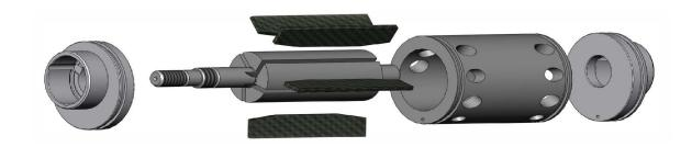
On the picture above you can see standard existing products on the market. It has stationary cylinder and lateral plates, and small openings with adhesive barriers among them for inlet and outlet from the working chamber.
